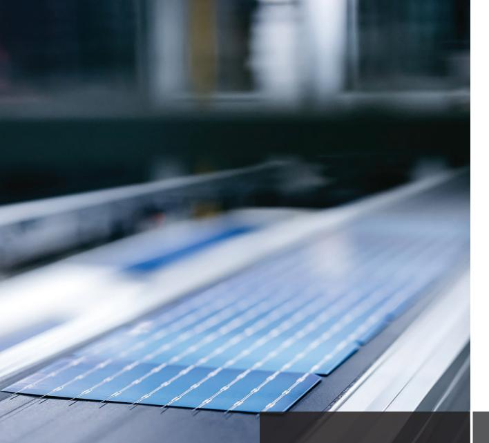
BISOL Duplex PV modules contain the most progressive M6 dimension half-cut cells (166 x 166 mm) and multi-busbar technology – both to maximise the energy yield to extremes.
