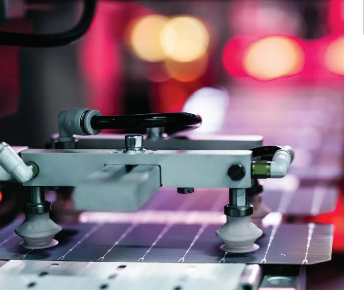
The tabbing stringing machines with laser cutters ensure non-destructive cell cutting for zero microcracks and power loss.
