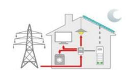
At night, when the energy stored in the battery is depleted, the public grid supplies energy to the domestic appliances.
