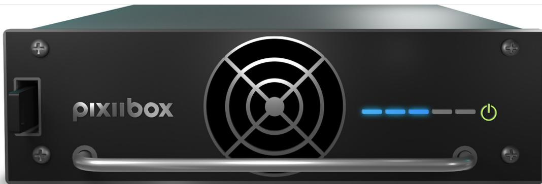
The PixiiBox is a fully bi-directional energy conversion module for energy storage systems. Operating as a rectifier, it can charge and maintain several battery technologies. Reversing the energy flow, operating as a grid tied inverter, it can feed energy back to the grid in accordance with international grid standards. The modularity enables scalability to match any power requirements from 3 to 300kW and an unmatched serviceability and reliability.
