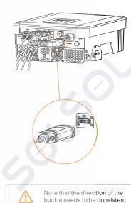
Connect the other side of the network cable to home router. And make sure the home router works in good condition.
