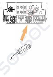
Plug the Pocket LAN into the correct port of inverter.
