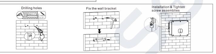
2.3 Installing the Monitor
