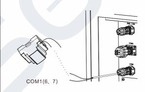
E. When connecting the smart meter to the inverter, connect one end of the cable to Terminal 13 (485B) and Terminal 14 (485A) of the smart meter and the other end to Pin 6 (485A) and Pin 7 (485B) of the COM1 port.
