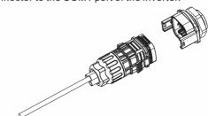
G. The standard RS485 cable length is 15m. If a longer RS485 cable is required, please use an intact cable and make sure the RS485 cable is less than 100m (the recommended length is less than 25m).
