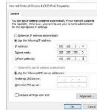
Figure 3- 1 Schematic diagram of static IP setting
