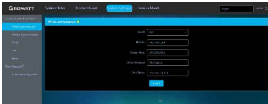
Figure 3- 23 Wired communication window
