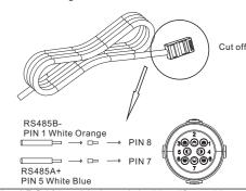
f.Plug the 8PIN signal connector to the inverter.
