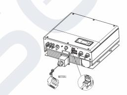
e.When you are installing a PV Inverter, first cut off the RJ45 modular plug, then find two cables and crimp the accessory terminals, finally, put them into the correspond interface
