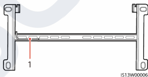
Figure 4-9 Position for binding the security Torx wrench
