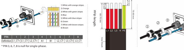
STEP 9: Insert the wires into the appropriate holes of the terminal STEP 10: Press the spring upward and push the base plate of communication board in. Then screw the countersunk screw.
