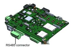
Figure 21: RS485 terminal block on the communication board
