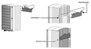
Figure 9: Hanging the inverter on the bracket
