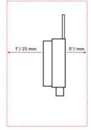
Figure 2: Power optimizer clearance
