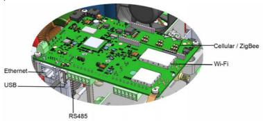
Figure 16: Internal connectors
