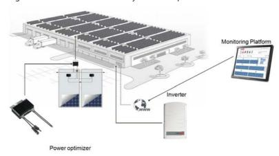
Figure 1: The SolarEdge power harvesting system components
