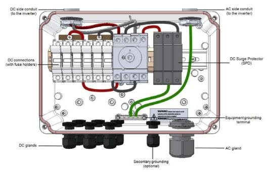
Figure 26: Inside the DC Safety Unit with fuses
