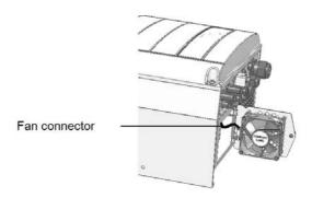
Figure 33: Fan connector
