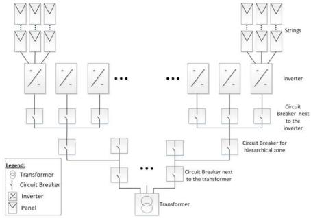
Figure 38: Typical transformer and commercial three phase inverter installation topology There are many considerations for selecting the suitable transformer and its associated current limiting devices such as circuit breakers and fuses. The considerations must include at least the following:
