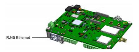
Figure 20: The RJ45 Ethernet connection
