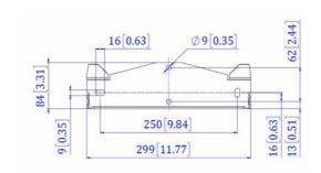
Figure 25: Inverter mounting bracket
