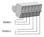
Figure 22: RS485 terminal block
