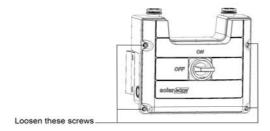
Figure 27: Opening the DC Safety Unit cover
