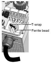
Figure 12: Attaching a Ferrite bead
