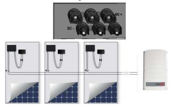
Figure 14: Inverter DC Connections
