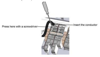
Figure 30: Spring-clamp terminals
